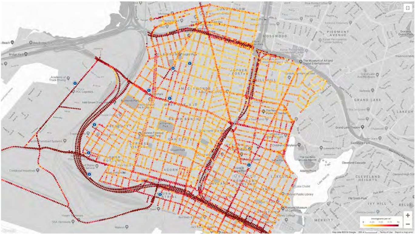
**BLACK CARBON MAP FROM THE ‘100X100 PROJECT’, A STATIONARY MONITORING NETWORK OF ONE HUNDRED AEROSOL BLACK CARBON DETECTORS DEPLOYED FOR ONE HUNDRED DAYS IN WEST OAKLAND.**
